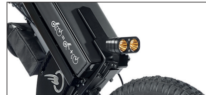
2000 lumens dual frontlight. Position and high beam lights. Retro-inspired yellow lens.
