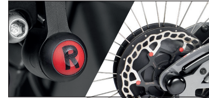
300 RPM 1200W high torque brushless motor with reverse gear. Maximum speed 30 Km/h.
