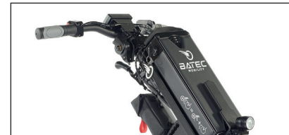
55 km* autonomy with 48 V - 768 Wh battery. Delivered with ultra-fast 3A charger.
