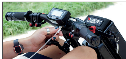
All-in-one LCD screen with gear selector. Horn and USB port.
