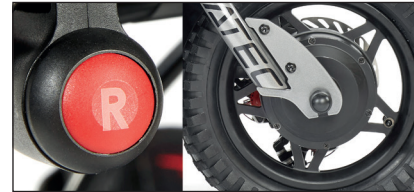
Brushless motor, 350 W nominal, 600 W maximum. Top speed of 20 km/h.
